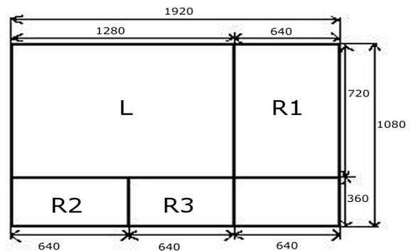
Since the two 720p video components have a frame rate of 50fps, the overall frame rate of the resulting composite video will be 50 fps as well. In some specific situations, however, lower frame rates might be also acceptable (24 or 25 fps).
