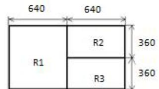
The three slices R1, R2 and R3 can be then inserted in the container frame as illustrated in the following figure.
